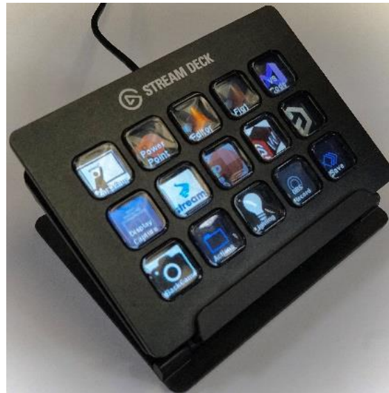
Figure 4: Stream Deck custom configured to automate operation of lightboard system
