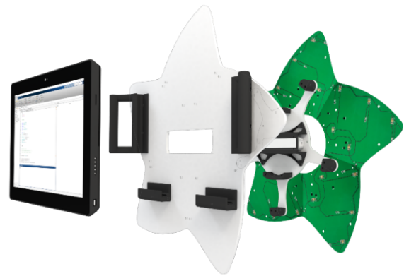
Fig. 1: Exploded diagram of 3D acoustic camera system developed in this study.
