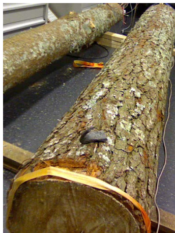
Figure 3: Photo log used for measurements with a transducer attached to the surface of the log using a strap.
