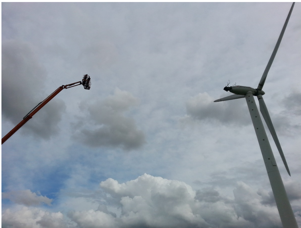
Fig. 5. Recording the sound at elevated position behind the turbine.
