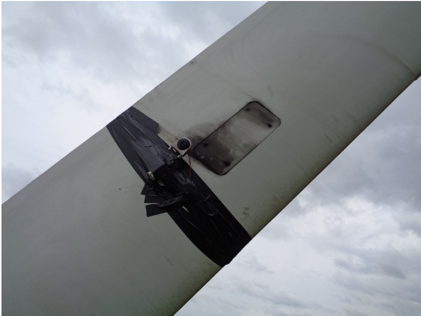
Fig. 8. Placement of a 2.5 kHz speaker on a turbine blade for Doppler shift experiment.
