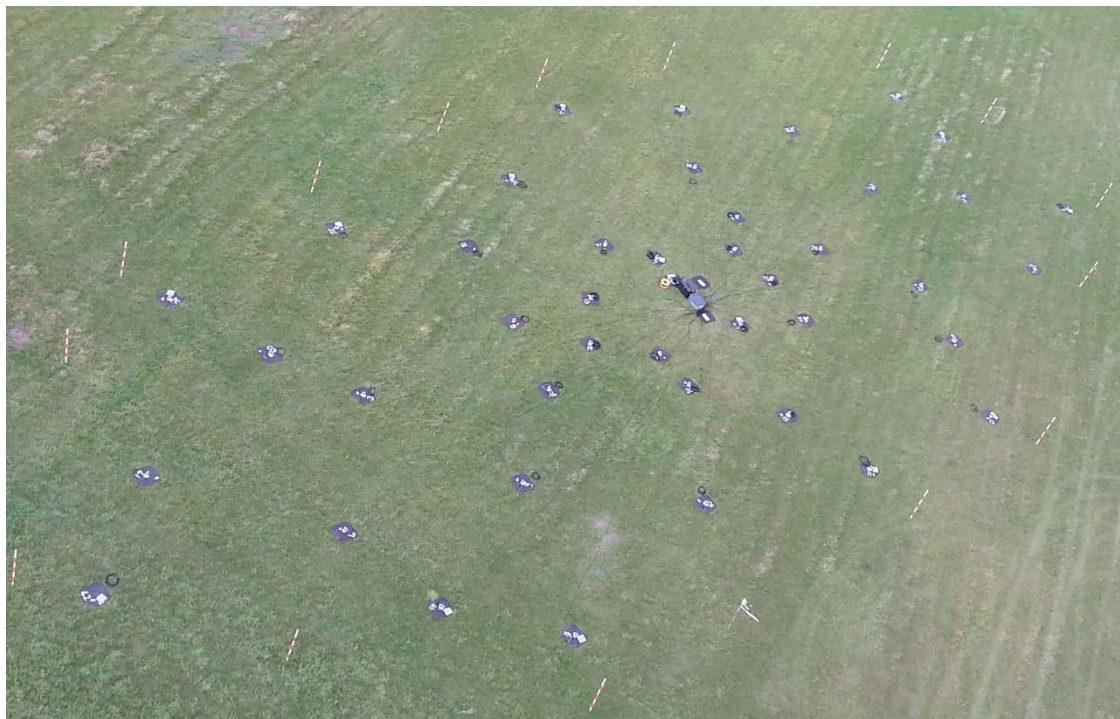
Fig. 3. View of the large spiral array from near the turbine hub height (the turbine is to the left of the camera position).
