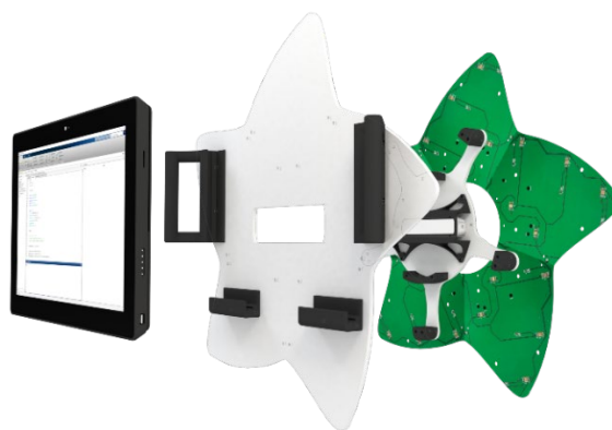
Figure 1. High level overview of acoustic camera used in this paper.
