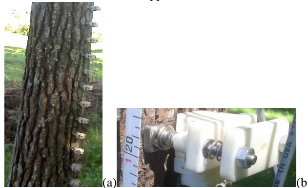
Figure 4: Photo (a) shows an array of transducers attached to a tree stem for measurement of same face and opposite face measurements. Photo (b) shows a close up of one of the transducers.
