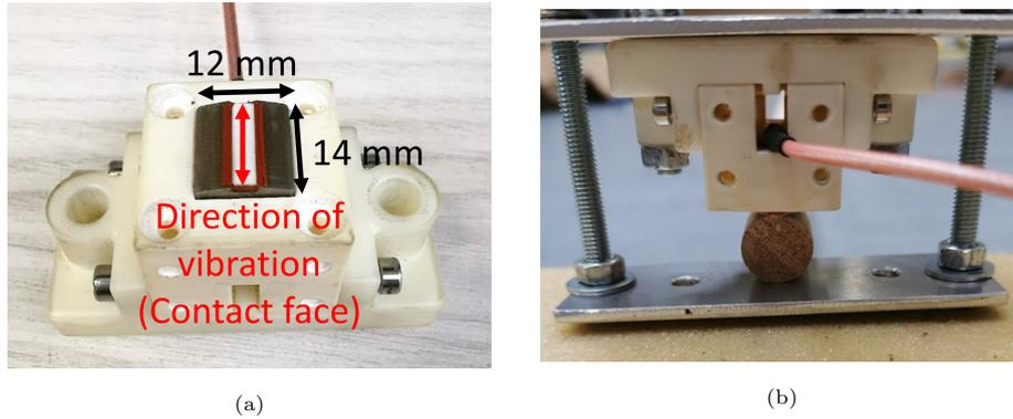
Figure 2: Photo (a) shows one of the shear transducers used in the experiment. Photo (b) shows the setup used to push a single transducer against the wooden sample.
