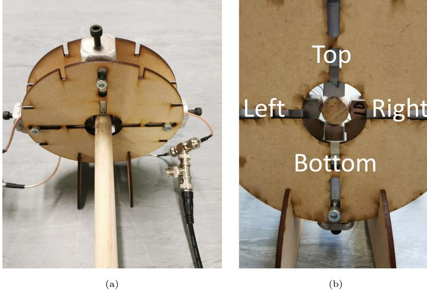
Figure 4: Photos of the transducer array mounting system used to position the transducers in a ring around the sample.
