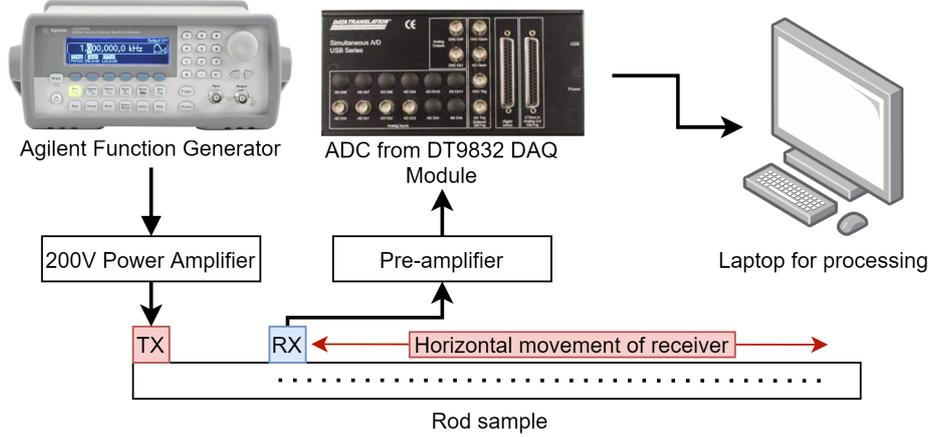
Figure 5: Experimental setup for obtaining the wavenumber plot
