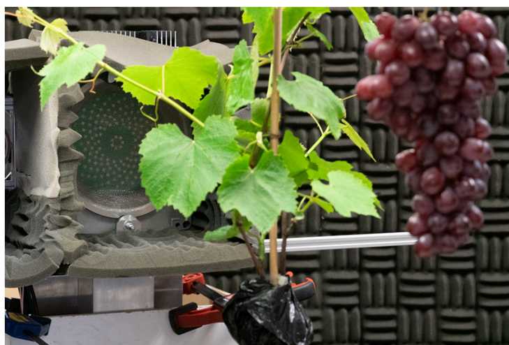
Figure 6. Photo showing the experimental setup with the grapes located behind a vine that is attached to a Computer Numerical Controlled (CNC) machine.
