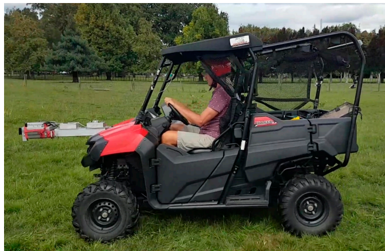
Figure 5. The farm vehicle with the ultrasonic pasture meter mounted on a frame and pointing downward at the pasture ahead of the vehicle. The ultrasonic pasture meter is at the front of the frame.
