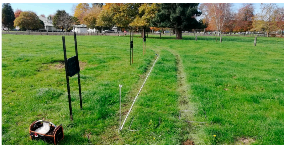
Figure 7. Transect 3 with three 0.5 m-wide reflectors. Ultrasonic profiles and biomass samples were taken from the start of the first post up to the last post. The 0.5 m \times 0.5 m quadrat frames can be seen.
