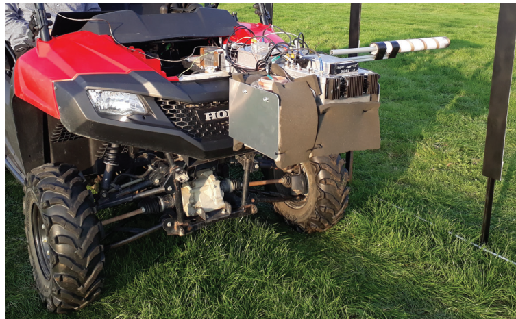
Figure 19. V1 and V2 arrays attached to a farm bike for field trials.
