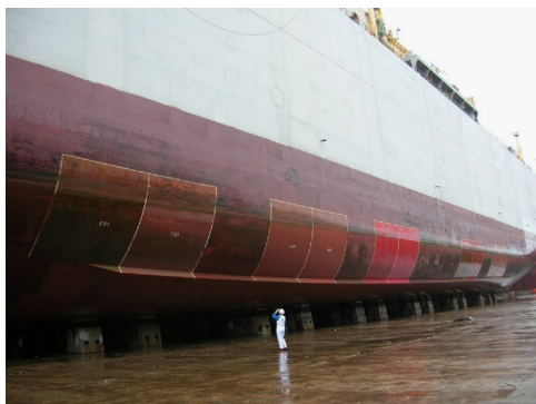
Fig. 1. Photo of a ship with antifouling coating on the hull. Photo provided by Lloyds Register.
