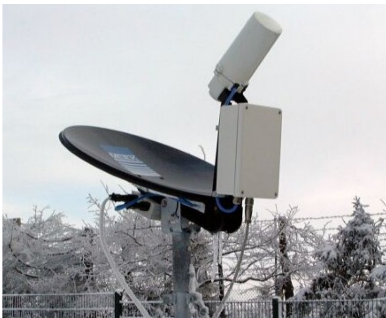
Figure 3.10: Doppler rain radar used in the evaluation of the sodar and fitting algorithm's ability to separate the rain component of the backscattered power spectra (Metek)
