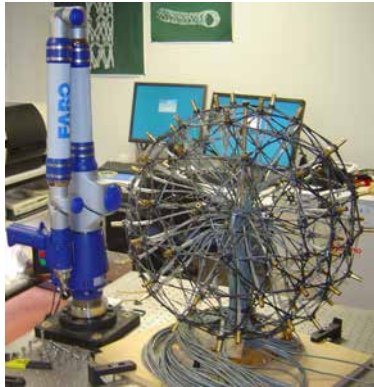
(a) Measurement of microphone coordinates using a Faro-arm.
