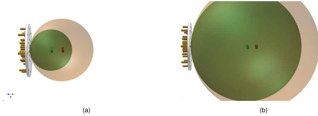
Figure 7.5: Diagram illustrating the difference in wavefront curvature for two sound sources separated by 50mm when they were at different distances from the array. Near the array distinct differences exist between the wavefronts arriving at the array from the two sound sources. However, as the sound sources are moved away from the array, the wavefronts become very similar. It is only by going to a larger array that differences in wavefront arrivals between microphones could be detected for the two sound sources.
