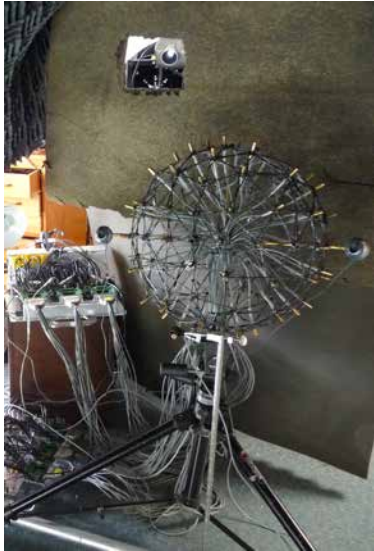
(a) Structured light setup. Three camera are attached to the spherical microphone array. A standard data projector is mounted to a stand behind and to the side of the array.
