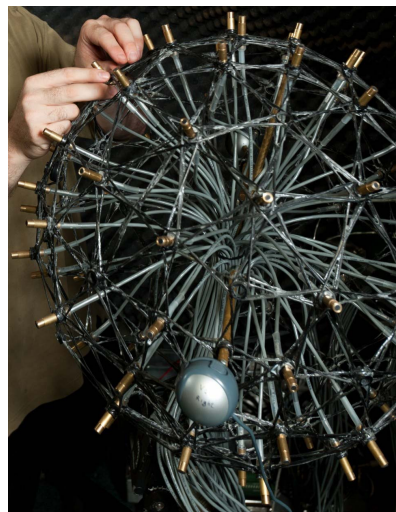
Fig. 1. Photo of a 72 element spherical microphone array containing three cameras which was used to test the calibration technique.
